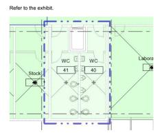
System Zones have been created in the model. A shape was used to define the Zone area using Sketch lines. As a result, extra spaces were selected that were not intended.
